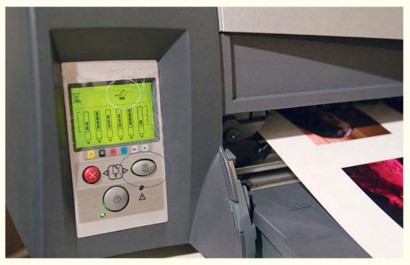
The icon of a finger on the HP Designjet 90 LCD screen signals that the print is finished. By pressing the button that is circled in blue, the print will eject. The amount of time which the print will pause before ejecting can be set in the printer driver.
