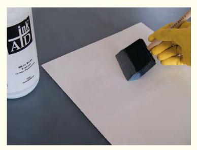
Applying the first coat of the inkAID White Matte Precoat onto a sheet of heavy art paper.
