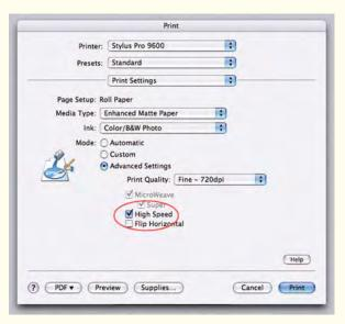
Edward Fausty's Epson printer driver settings, used when making prints on uncoated fine art papers over 13×19 inches. The High Speed box is circled in red. This makes the printer print in bi-directional mode, which is faster than uni-directional mode (unchecked).
