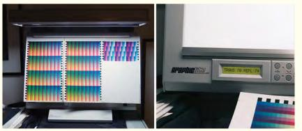
(Left) Douglas Dubler's GTI SOFV-1e viewing system in reflective mode with three profiling target charts, output through the SpectralVision Pro software accessible from within the ColorBurst X-Proof RIP. (Right) The digital readout of the SOFV-1e, showing the current intensity level of the transmissive and reflective light.
