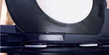
A Canon imagePROGRAF iPF5000 on a table with furniture sliders under four corners (two shown) to allow the printer to be easily rotated if necessary. The primary reasons for rotating the printer would be to change roll paper or to feed a thick sheet from the back of the machine.
