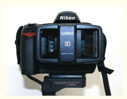
The Loreo Stereo Lens-In-A-Cap (T) mounted on a Nikon D70. Photo © Bonny Lhotka
