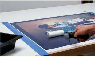
(Left) Patrick Carr taping down a canvas print with blue masking tape prior to coating. (Right) Patrick Carr demonstrating how he applies the varnish using a six-inch-wide short-napped paint roller.
