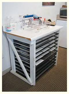
Darkroom print drying rack being used to allow inkjet paper to dry and flatten out.
