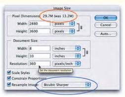
(Left) Photoshop's Image>Image Size dialog box before interpolating, and with Bicubic Smoother selected. (Right) The Image Size dialog box after upsizing by 50% (note the change in file size—circled in red).
