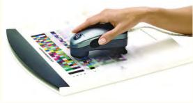
(Left) A profiling target being read with an i1PRO Spectrophotometer and ruler with a few sheets of paper under it. (Right) A similar profiling target being read using an i1PRO, newer version of the ruler, and X-Rite's i1 foldable backing board. (Left) Photo © Andrew Darlow (Right) Image courtesy X-Rite
