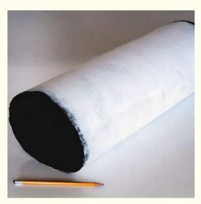
(Left) Precoated paper hanging to dry from binder clips. (Right) Precoated paper rolled in a loose cylinder to smooth out remaining wrinkles.
