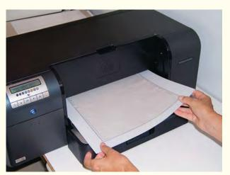
Loading the paper attached to the carrier sheet into the HP Photosmart Pro B9180's manual feed tray. Photo © Karin Schminke
