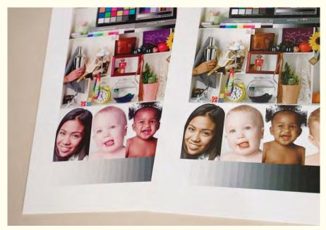
The inkjet print on the left was output incorrectly with settings that caused "double profiling." The print to the right was output properly using the same paper, and on the same printer.
