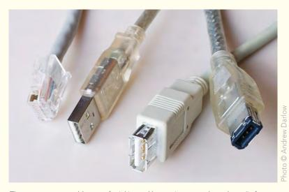
The most common cable types for inkjet and laser printers are shown here. (Left to right) Ethernet Cat. 5e connector, USB connector for the computer (the other end, for the printer, is square), a USB extension cable connector, and an IEEE 1394 connector (a.k.a. FireWire).
