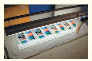
A simple fluorescent light-testing setup with multiple copies of the same image, printed on multiple papers and with multiple printers. The print samples shown are covered with standard window glass to reduce airflow over print surfaces, thereby eliminating one of the print-fading variables. Photo © Harald Johnson.
