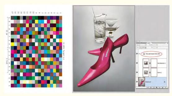
(Left) A CMYK target file included with X-Rite's i1Match software. (Right) After soft proofing using the CMYK profile created from the printer's proof, two adjustment layers were created to increase contrast and improve the look of the saturated pink color of the shoes before converting the file to CMYK.
